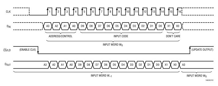
Figure 1. Register Loading Sequence
